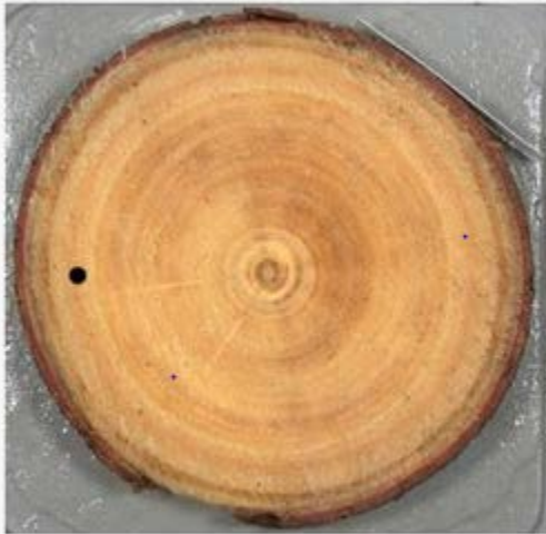
Sectioned disc scanned using colour and X-Ray imagery
