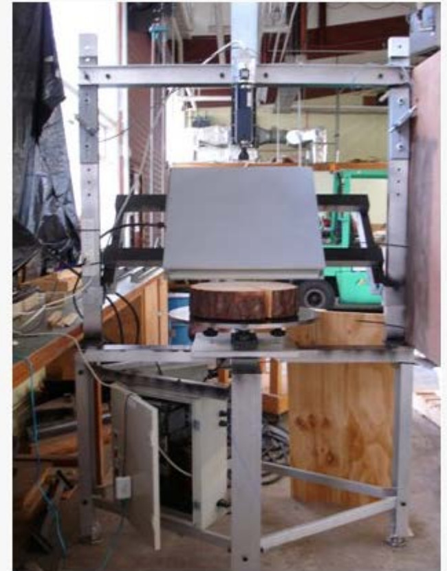
Scanning disc using Near Infrared (NIR) Robot
