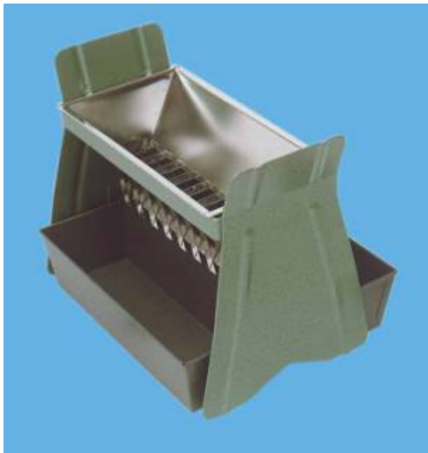
Figure 2: Example of mechanical sample dividers of the 'multiple slot' type (riffle box).
